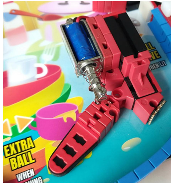
Fig. 5: A solenoid as a flipper driver.
