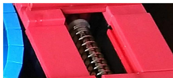
Fig. 6: Detail of plunger spring with washer.
