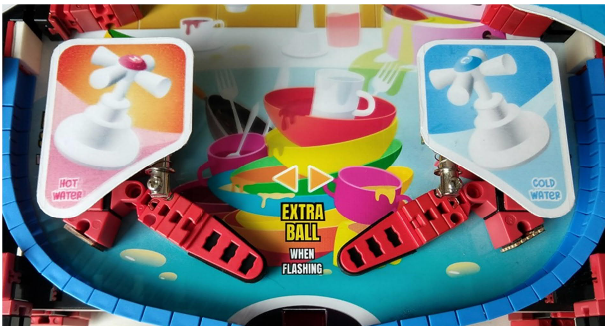
Fig. 1: Front view of the “Dirty Dishes” pinball table. The solenoids that activate the flippers are below the pink and blue covers.
